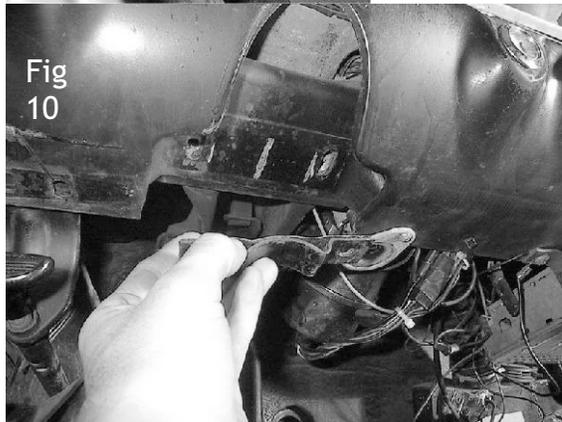
14. Slide the firewall bracket onto the end of the column then replace the upper half of the stock column clamp (Fig 10) and install the column using the supplied bolts. Do not tighten until after u-joint assembly is installed. Use factory rubber seal at the firewall.
