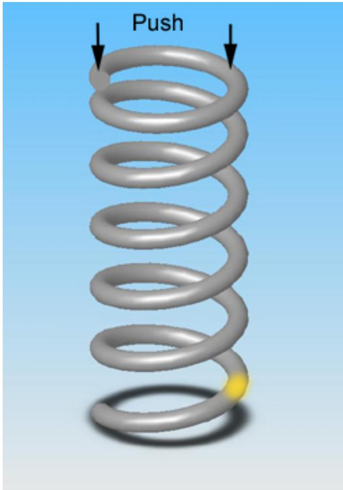
Quickly flip the spring and push the newly cut end against the shop floor to set the end so it will fit the pocket. Keep it vertical so the end forms flat for the pocket. **DO NOT quench the spring in water**, rather let it air cool slowly.
