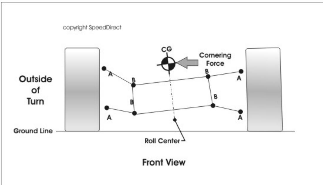
As you can see starting with positive camber sets the car up to maximize contact patch in a turn. The opposite is true if for some strange reason you started with negative camber. With negative camber as the suspension is loaded, and the car rolls (leans) the tire would not remain flat and thereby lower available traction.
