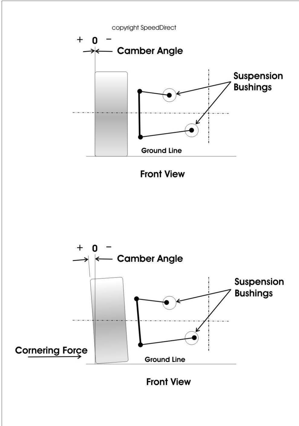
Another steering input in which squishy bushings can change steering angle as you enter a corner is deflection steering. This is a bad side effect of having a flexible bushing in the system. Deflection steering can take two forms; deflection oversteer or deflection understeer depending on how your car's steering is designed. If the steering link in front of the axle (front steer) it can cause understeer or the tendency to widen the radius of the intended
