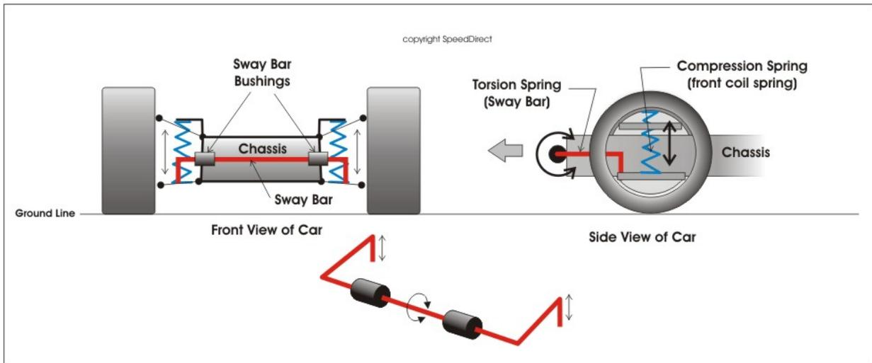
Body roll is also connected to whether a car has bad habits like oversteer previously discussed. That's because the more the body rolls the more it messes with the steering geometry (mostly camber) causing the car to do things you would not expect when you corner. We have shown the front
