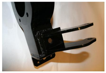
3. Weld all edges of the bracket to the trailing arm.
