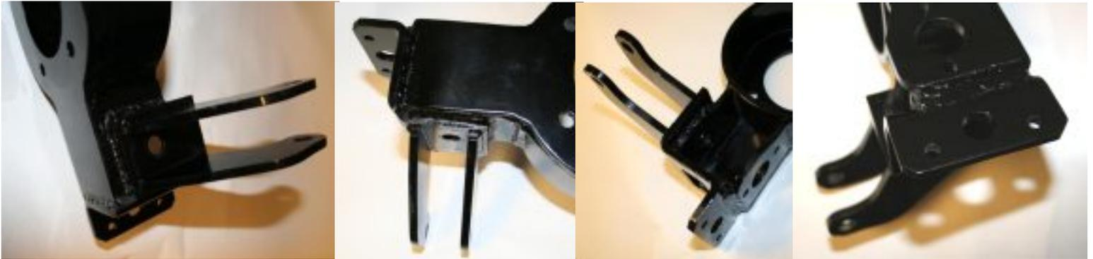
*Photos taken after welding and powder coat.*
