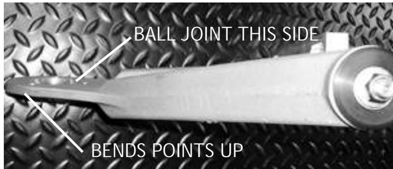
This view is of the passenger side a-arm viewed as if you were looking toward the back of the car. Notice that the end where the ball joint attaches is bent up.
