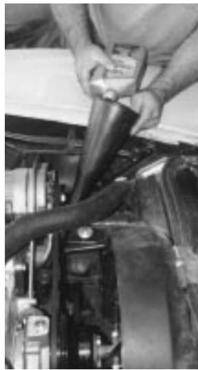
Fluid is then added to the system to bring the level to the appropriate mark ("cold," in this case)...
