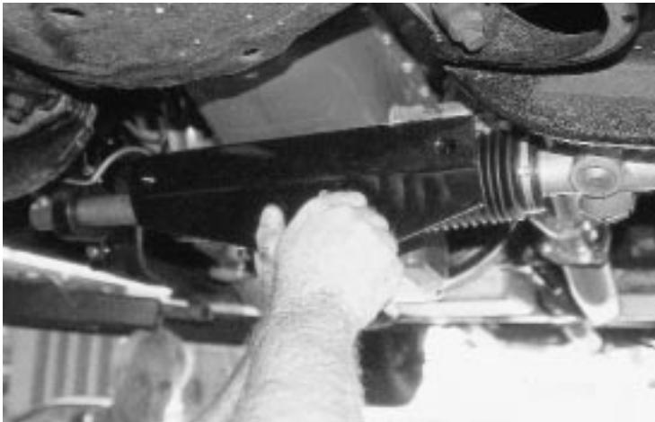
The next step is to bolt the tie rod bracket to the rack-and-pinion. The outer holes are positioned to the top of the rack.
