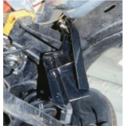
The passenger-side bracket for the new set up bolts in just as the old idler arm did.
