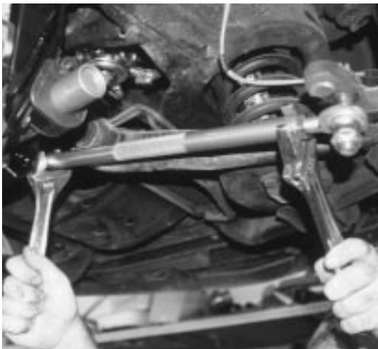
Coming into the home stretch, Loy used a pair of adjustable wrenches to set an approximate alignment. Since Auto Perfections has an alignment rack, the '72 didn't have to travel far to get the job done correctly. For the rest of us, the Steeroids™ instruction sheet outlines a procedure for setting an approximate alignment.
