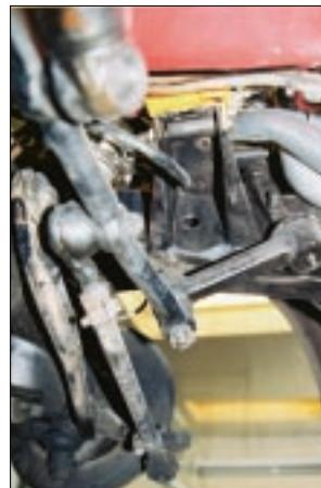
Once all that's done, you'll end up here—at the passenger-side idler arm. After making sure someone is supporting the system, remove the two bolts holding the idler arm to the frame, and the last bolt securing the steering box. The entire system can then be removed from the bottom of the car.
