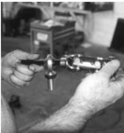
The intermediate shaft support bearing can then be installed onto the remaining part of the assembly.
