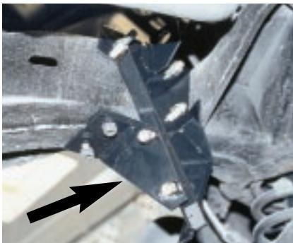
Moving to the left side, the new driver-side bracket bolts in at the same location as the old steering box. The Steeroids setup also includes a driver-side gusset, which attaches to the mount for the power assist cylinder (arrow).
