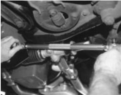
After threading the new tie rod ends onto the supplied tie rod sleeves, the two tie rod assemblies are bolted to the tie rod bracket and each side's steering knuckle. Be sure to tighten both castle nuts so that new cotter pins can be installed.
