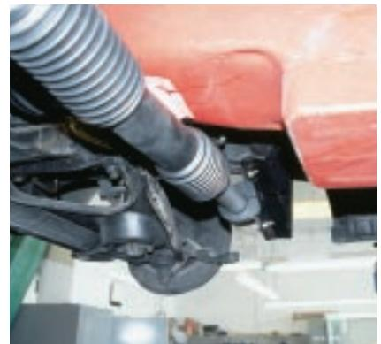
The rack-and-pinion is then mounted to the frame brackets that were previously installed and torqued to the specified value (30 ft-lbs, in this case).
