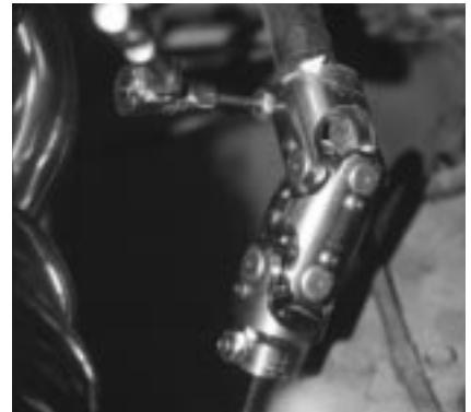
The U-joints are secured to their respective shafts with set screws. The steering column set screw should sit on the flat, machined surface before its tightened; the other set screws will need to be aligned with matching holes in the Steeroids™ shafts. Be sure to use a little thread-locking compound on the set screws.
