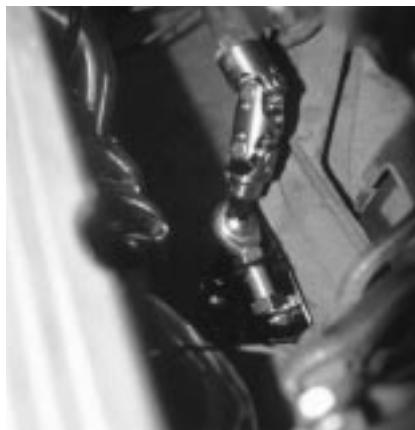
As seen here, the double U-joint connects to the factory steering column, while the intermediate shaft has been reconnected to the single U-joint. The support bearing bolts to the driver-side bracket.
