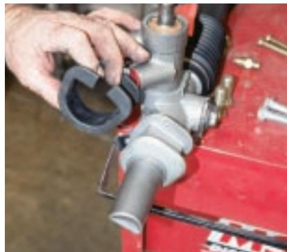
These two large, rubber split-bushings are then installed onto the rack-and-pinion unit. The shape of each one corresponds to its mounting surface on the new rack, making this a foolproof operation.
