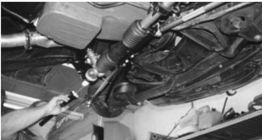
...after which the car can be started and a thorough check for leaks made. Everything was fluid-tight. The only thing left at this point is to get the Vette's front-end precisely aligned—and then to enjoy the car's slop-free rack-and-pinion steering.
