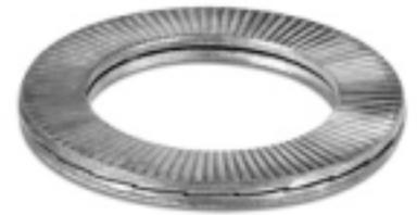
NORD-LOCK is a pair of washers with a wedge-locking action meeting DIN 25201 which is a unique method using tension instead of friction. The rise of the cams between the NORD-LOCK washers is greater than the pitch of the bolt. In addition, there are radial teeth on the opposite side. The washers are installed in pairs, cam face to cam face.
