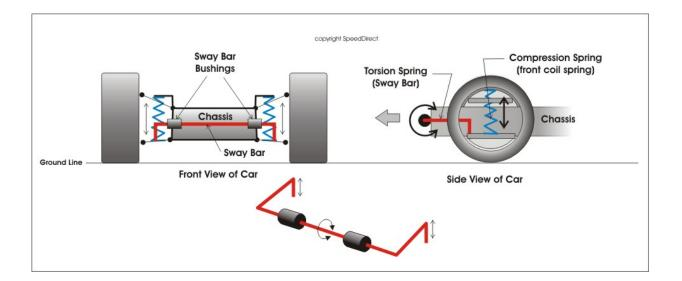
Body roll is also connected to whether a car has bad habits like oversteer previously discussed. That's because the more the body rolls the more is messes with the steering geometry (mostly camber) causing the car to do things you would not expect when you corner. We have shown the front
