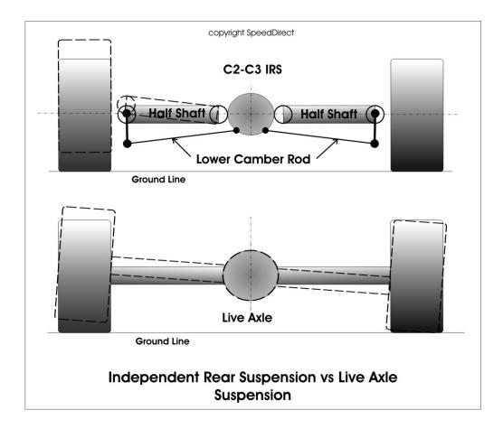
Along with this great ability to follow the surface better there are some deficiencies associated with the basic design of the system. All IRS systems are not alike and Corvette has some unique features which can cause head aches for some one wanting good cornering performance in all conditions.
