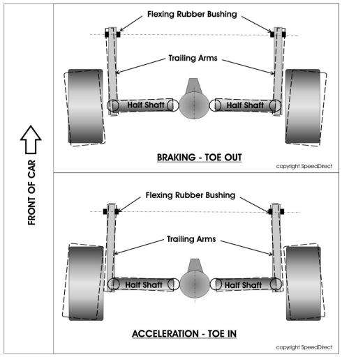
C2-C3 IRS Torque Steer (Top View)
