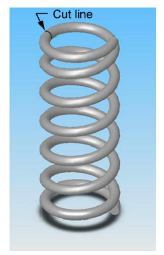
Cut the spring with an oxy acetylene torch on the mark.
