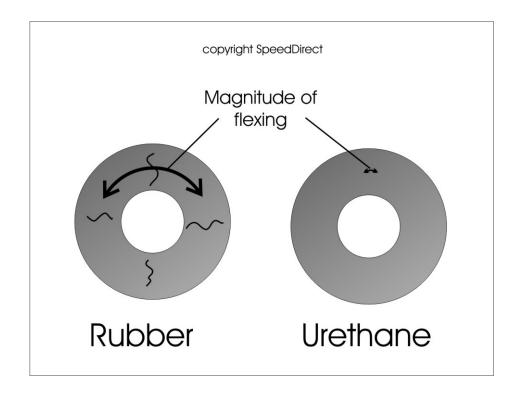
On the SpeedDirect upper a-arm alloy a-arm for C2-C3 Corvettes we chose rigid composite bushings which are Teflon impregnated to eliminate all of the described problems of bushings. They are stiff, do not flex, they run smooth on the cross shaft, and need no lubrication for the life of the installation.
