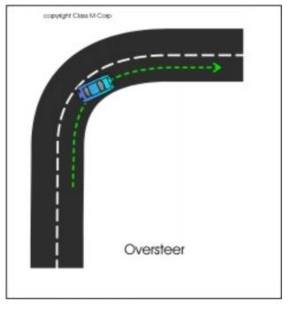
Symptom - You turn and the front end has greater traction than the rear and the rear end swings out in the direction of the corner.
