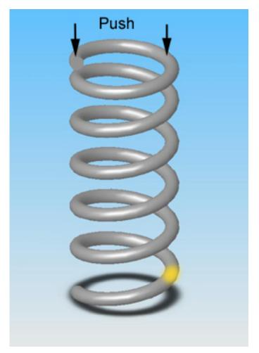
Quickly flip the spring and push the newly cut end against the shop floor to set the end so it will fit the pocket. Keep it vertical so the end forms flat for the pocket. **DO NOT quench the spring in water**, rather let it air cool slowly.
