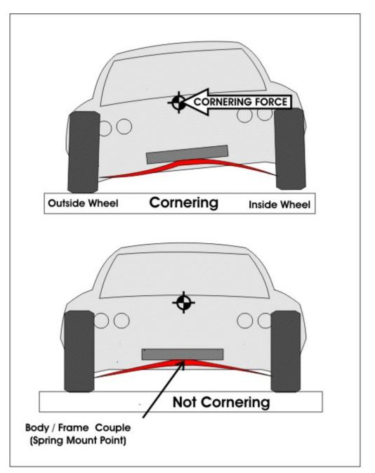
The Shark Bite rear coil over design offered by SpeedDirect for the C2-C3 Corvette is great way to sever the tie between both sides and restore true independence. It is also designed with quick release pins to enable both springs to be changed in about twenty minutes! We believe this arrangement, plus the adjustability mentioned gives a performance driver the most flexibility in setting up the car to handle beyond what is possible with a transverse leaf spring.
