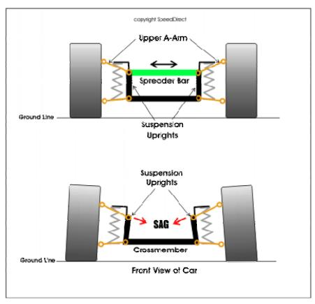
A spreader bar will push; spread, the sagging upright mounts back to their proper upright position. The front suspension will then be back to where it was designed to be positioned, and will resist flexing associated with cornering. By "boxing" the front end with an additional member (the spreader bar) overall stiffness is greatly increased. The car will hold its intended alignment and camber closer to what it needs to be to corner and handle consistently.
