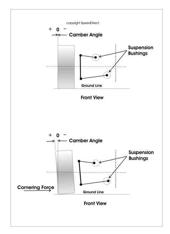
Another steering input in which squishy bushings can change steering angle as you enter a corner is deflection steering. This is a bad side effect of having a flexible bushing in the system. Deflection steering can take two forms; deflection oversteer or deflection understeer depending on how your car's steering is designed. If the steering link in front of the axle (front steer) it can cause understeer or the tendency to widen the radius of the intended
