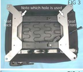
\*The rear floor brackets can vary in shape depending on year of Corvette. '74-'82 bracket assembly shown.
