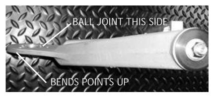
This view is of the passenger side a-arm viewed as if you were looking toward the back of the car. Notice that the end where the ball joint attaches is bent up.
