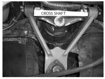
This view is of the passenger side control arm shows the installation of the cross shaft with the tapered end (as viewed from above) facing the front of the car.
