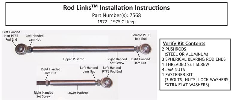
One or more of the bearing ends are PTFE-lined, which require no lubrication. This can make them difficult to turn by hand. This tight fit keeps debris and dirt out of the bearing race and essentially makes them self-cleaning.
