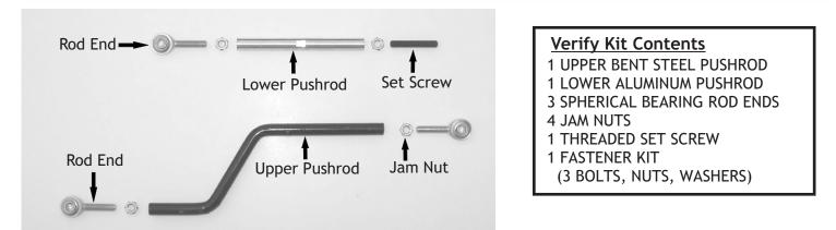
One or more of the bearing ends are PTFE-lined, which require no lubrication. This can make them difficult to turn by hand. This tight fit keeps debris and dirt out of the bearing race and essentially makes them self-cleaning.
