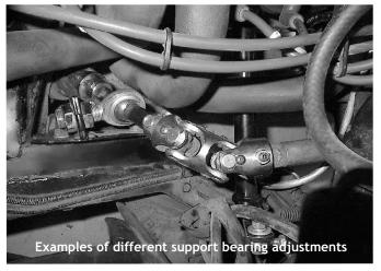
be sure the support bearing is loose during adjustment. After all other items are tightened, re-tighten the jam nuts on the support bearing. Additionally, check the condition of the steering column bearing located at the end of the column tube. If it shows signs of play, it is recommended that it be replaced since a loose bearing can cause u-joint binding and excess play in the steering wheel.
