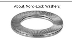
NORD-LOCK is a pair of washers with a wedge-locking action meeting DIN 25201 which is a unique method using tension instead of friction. The rise of the cams between the NORD-LOCK washers is greater than the pitch of the bolt. In addition, there are radial teeth on the opposite side. The washers are installed in pairs, cam face to cam face.
