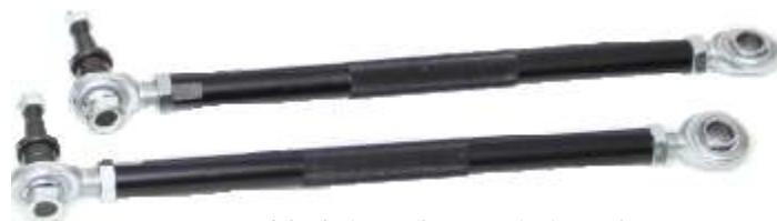
Assembled tie rods, consisting of: 690-72657 tie rod sleeves 690-56515 tie rod ends 690-50067 (2 smaller bearings from kit)
