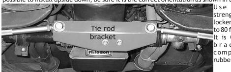
Use a highstrength thread locker and torque to 80 ft/lbs. It is OK for the bracket to compress the rubber boot.
