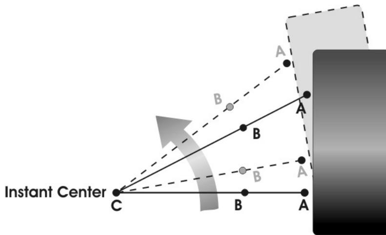
Drawing another line from the centerline of the bottom of the tire, point E to the instant center, point C and still another set for the other side of the suspension will give you the roll center. It is the point where these two lines meet. The height of the roll center is measured from ground level.
