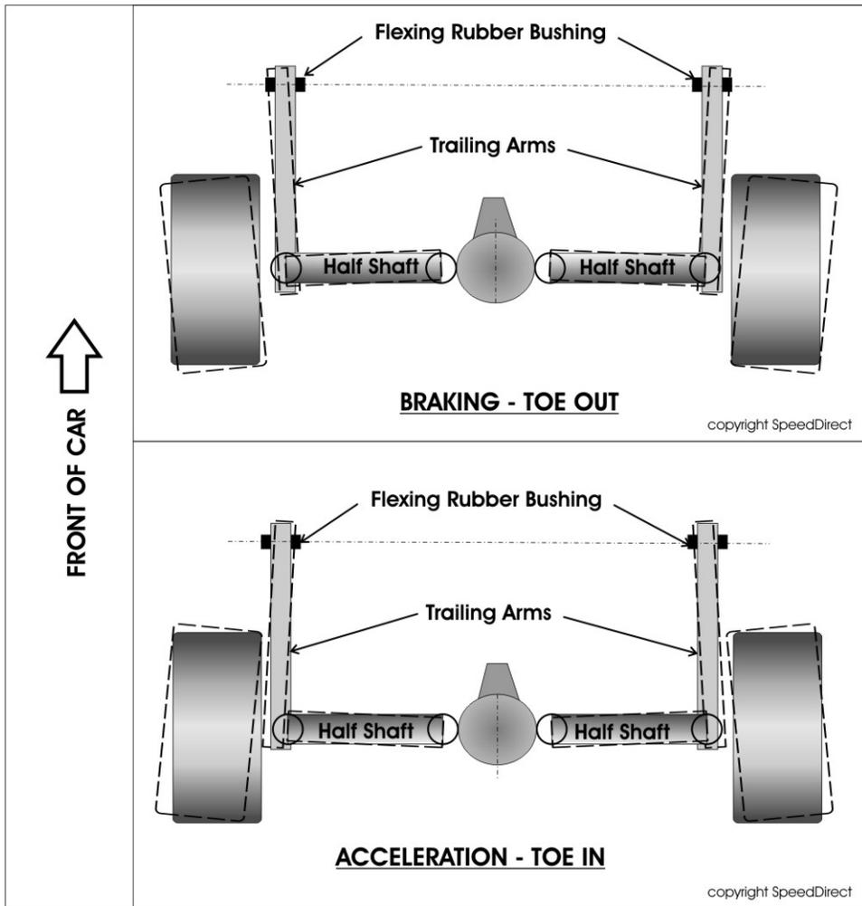
**C2-C3 IRS Torque Steer (Top View)**
