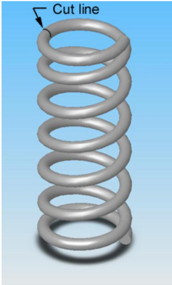
Cut the spring with an oxy acetylene torch on the mark.
