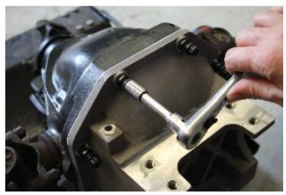
5. Install new gasket and new cover. Tighten all bolts evenly and then torque to 50 ft/lbs. **Stock only:** All the bolts are the same length. **Shark Bite only:** If installing a cover with an integrated lower shock mount for Shark Bite rear coil-overs, use the provided 1.75" long 12-point bolts in the two lower holes (these bolts are included with all Shark Bite kits).
