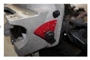
on the ends of the support struts may be needed (Fig 1). Place the supplied washers between the strut and the cover.
