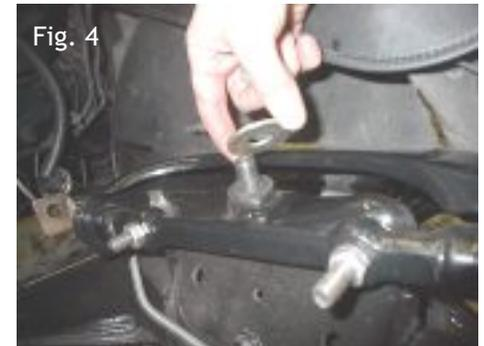
8. From the top of the shock remove the nut, one washer and one bushing. Leave the other bushing and washer on the stud. Be sure that the shock is fully extended.
