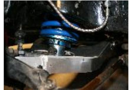
**PLEASE NOTE:** These shocks feature a small hydraulic bypass that allows them to be extended and compressed by hand. The actual shock valving does not begin to work until the velocities are higher than what can be applied by hand. Therefore, you will not be able to notice a change in stiffness when you change the valve settings and operate the shock by hand.
