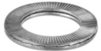
NORD-LOCK is a pair of washers with a wedge-locking action meeting DIN 25201 which is a unique method using tension instead of friction. The rise of the cams between the NORD-LOCK washers is greater than the pitch of the bolt. In addition, there are
