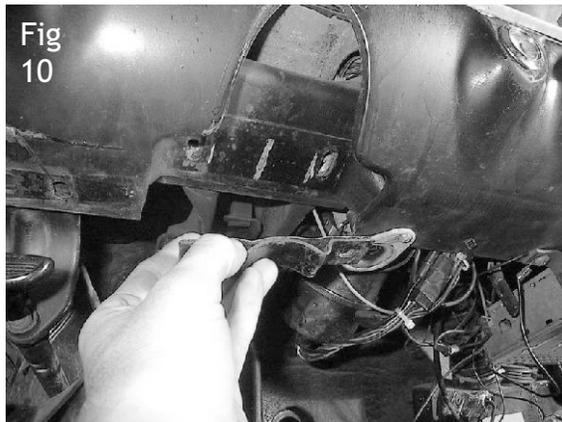
14. Slide the firewall bracket onto the end of the column then replace the upper half of the stock column clamp (Fig 10) and
