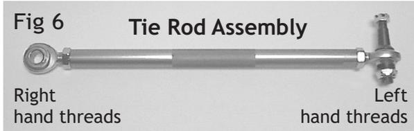
10. To set an approximate alignment, measure the overall length of the old steering system, measuring it from the center of each outer tie rod end. Adjust the tie rods on the steering rack to match the measurement and tighten the jam nuts against the sleeves.
